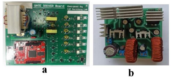
Fig. 8. the prototype of the proposed converter (b) and controller circuit (a)
