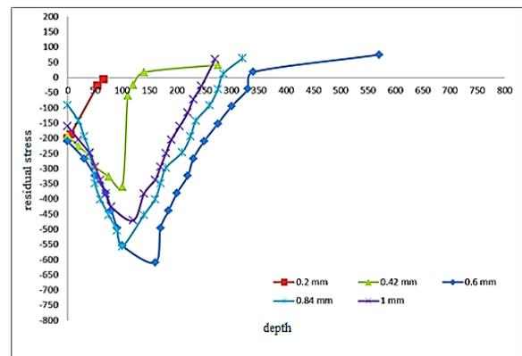
Fig.8. Influence of shot diameter on the residual stress profile
